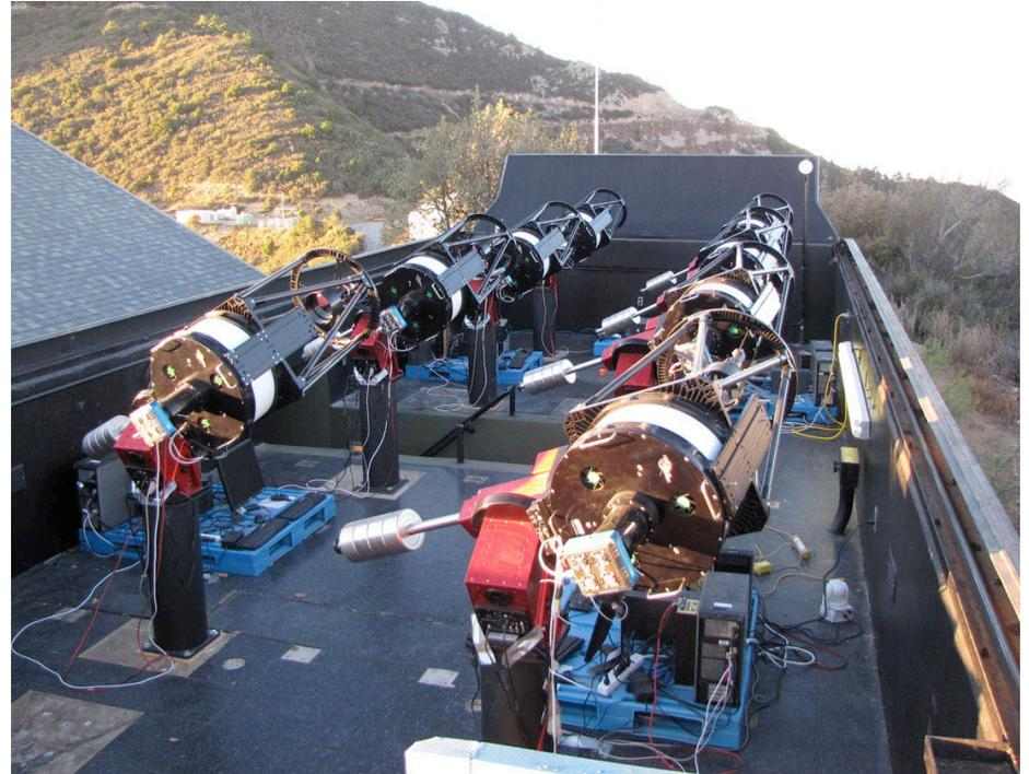
*Eight 16" telescopes monitor a few thousand stars cooler than the Sun, searching for transiting planets as part of the MEarth project. Similar ground-based configurations may soon be able to detect Earth-sized planets. Image from Dan Brocius.*
